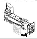
Un-clip the Wall Plate Cover and slide down the arm.
