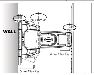
Step 8. Adjust tilt and roll if necessary
