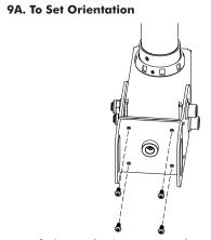
1. Loosen the 4 screws using the supplied 2.5mm Allen Key.
