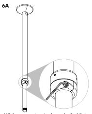
Whilst supporting the lower half of Pole Assembly loosen the Socket Cap Screws (x2) using the supplied 5mm Allen Key.
