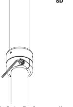
Tighten the Socket Cap Screws (x2) to set the height using the supplied 5mm Allen Key.
