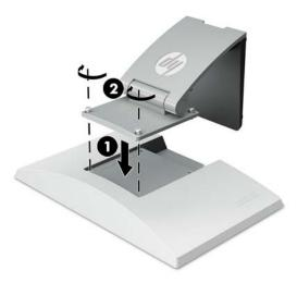
3. Tilt the stand back to access the bottom of the mounting plate.
