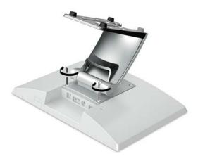
5. To route cables with a stand attached, snap off the routing cover on the neck of the stand (1). Route the cables down the neck of the stand, and then through the hole in the center of the base and out the underside of the base (2). Snap the cable routing cover onto the neck of the stand to cover the cables (3).
