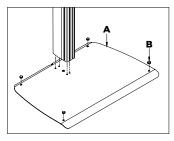
Optional: Bolting the Stand to the floor Remove the hole caps (part 2) and adjustable rubber feet from the floor plate (part 1). Pre-drill holes in floor and using suitable ground anchor fixings (not supplied), fix stand to floor.
