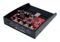
The 35BAYUSB3S4 3.5-inch Front Bay to 4-Port USB 3.0 Panel Hub turns any available 3.5-inch computer case front bay into a 4-Port USB 3.0 hub.
