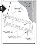
TIP: Use a spirit level to ensure the wall plate is horizontal
