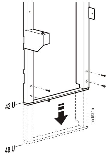
4. Place the mounting frame onto the enclosure.
