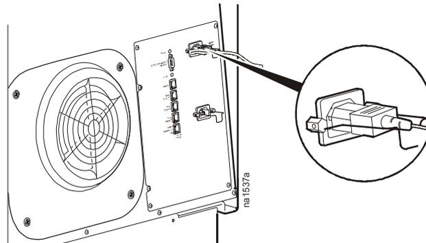
3. To provide redundant power to the unit, use the **B** input socket to connect the ARU to a second source of protected power.
