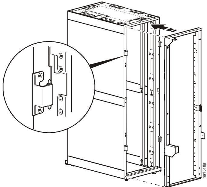
3. Secure the frame to the enclosure using six M6 Phillips screws.
