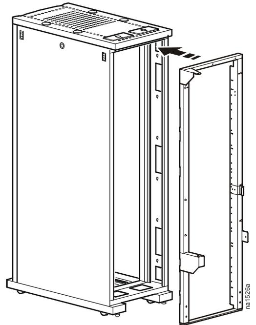
2. Secure the mounting frame to the enclosure using eight M6 Phillips screws (four per side). Use the holes marked **C** on the inside edges of the mounting frame.
