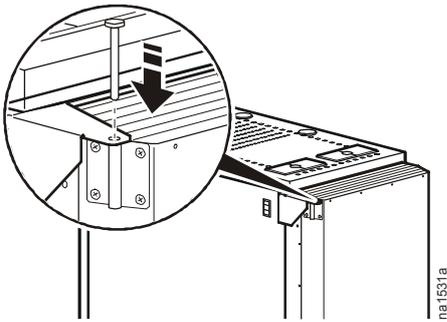
4. Align the upper hinge of the mounting frame with the upper hinge of the fan assembly, and slide the hinge pin into position.
