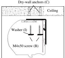
NOTE: The brackets do not slide. They are designed to attach the end caps only.
