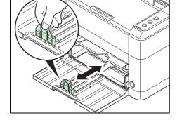
**Note** When using paper larger than A4/Letter, pull out the paper length guide.
