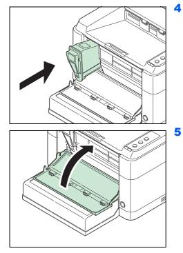
Install the new toner container in the printer. Push in firmly until you hear a "click" sound.
