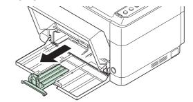
When using A6 paper, attach the stopper.
