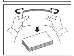
If the paper is curled at an edge, straighten it prior to reloading.
