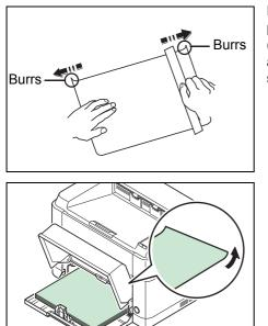
Fan the stack of paper and align the edges before loading them in the paper source. Some types of paper have rough edges on the back (those are created when the paper is cut). In this case, put the paper on a flat place and rub the edges once or twice with, for example, a ruler to smooth them. Feeding rough edged paper may cause paper jams.
