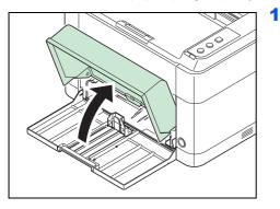
**Note** When using paper that is larger than A4/Letter, remove the cassette cover. Gently press on both the left and right sides of the cassette cover and pull.
