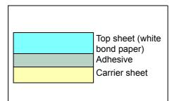
Label paper has a structure comprising of three layers, as shown in the diagram. The top sheet is printed on. The adhesive layer consists of pressure-sensitive adhesives. The carrier sheet (also called the linear or backing sheet) holds the labels until used. Due to the complexity of its composition, adhesive-backed label paper is particularly likely to give printing problems.
