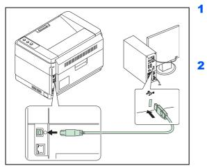
Connect the USB cable to the printer's USB interface connector.
