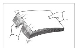
**3** Remove all the even pages (including the instruction sheet) from the output tray, fan through the sheets to separate them prior to loading.
