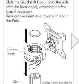
Slide the Quickshift Donut into the desired position. If necessary, adjust the tension between the Quickshift Donut and the Pole using the 5mm Allen Key supplied.
