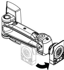
Un-clip the Wall Plate Cover and slide down the arm.
