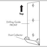
Drilling Guide BACK 0 0 Double-sided tape (x2)
