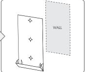
Peel away the backing from the double-sided adhesive tape.
