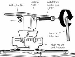
Tip: When the projector requires servicing, remove the projector via this easy disconnection point to save time.
