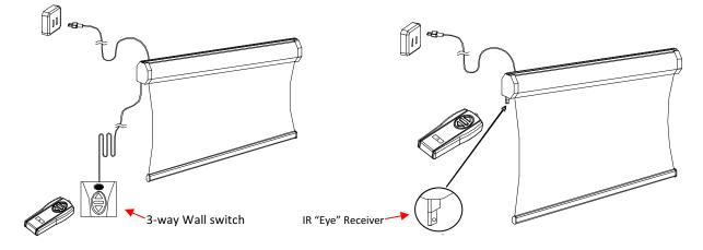
**4. IR Remote Control:** The Infrared functions by direct line of sight contact with a beam range of 30 feet.
