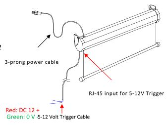
**2. 3 -Way Wall Switch:** The 3-way wall switch is a wall mount control box with an up/stop/down button and plugs directly into the screen's RJ-45 input.
