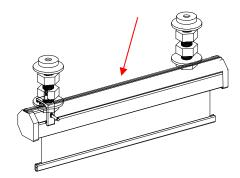
2. Slide the **Extruded Hanging Bracket (D)** through the rail located below the slide channel until it meets with the top of the **Bolt (B)** and slightly secure the lug-nuts located on the top & bottom of the bolt to attach the bracket.
