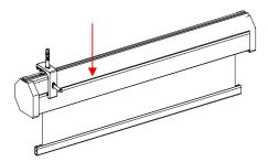
3. Mark the installation location to drill your hole. Insert the proper screw and secure the bolts to the bracket.
