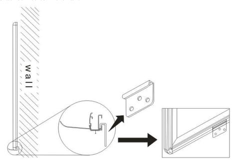
4. Drill and insert the **hollow wall anchors** (c) into the drilled holes, and then screw the bottom hanging bracket to wall.
