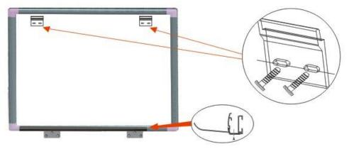
2. Next, attach the **tray** (i) to the bottom of the WhiteBoardScreen Universal with the three **M5 screws** (h) as shown below.
