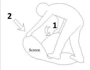
2) While holding the material down with both feet, lean forward and grab the left and right side.
