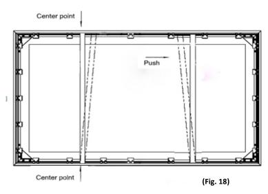
3. Slide the top end of the bar into the top center point of the frame to complete the center support bar installation. This will provide added stability to your frame and added tension to the material.
