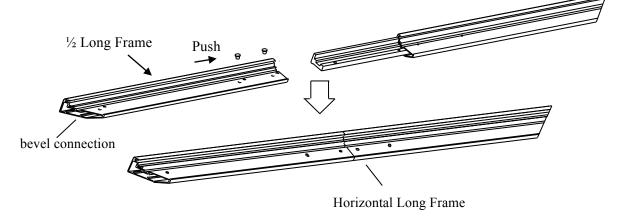
Note: a. 2 long frames should be assembled for a screen.
