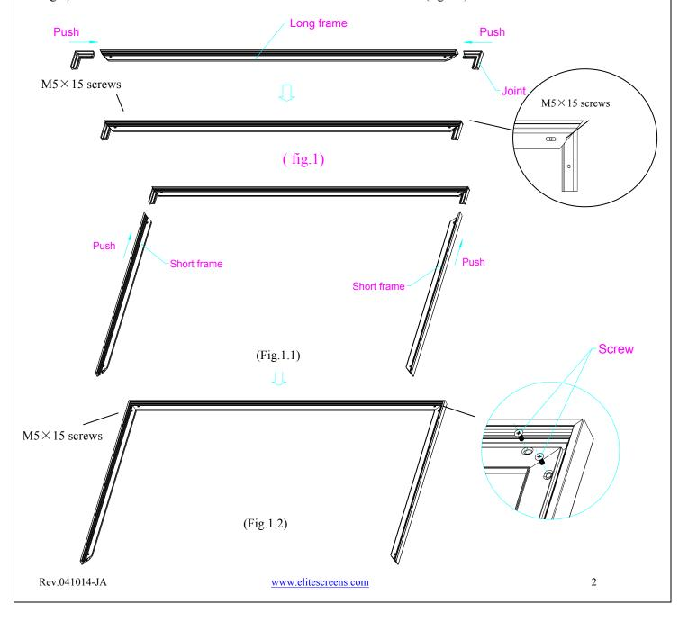
Join all four frame parts together following the steps shown below. (Fig.2)
