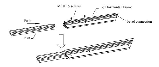
2. Insert the other 1/2 horizontal frame piece to the **center joint** connector and fasten it with two **M5x15 screws**. Repeat steps 1 and 2 for assembling the second horizontal frame.
