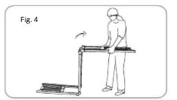
2. Unfold the frame until the latch on the hinge "clicks" into place. Repeat the procedure for the shorter
