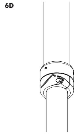
If necessary, centralise the Pole Joint by tightening the Set Screws (x2) to suit using the 2.5mm Allen Key.
