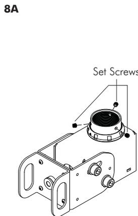
Loosen the three set screws using the supplied 3mm Allen Key.
