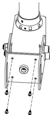
1. Loosen the 4 screws using the supplied 2.5mm Allen Key.
