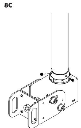
Secure the collar with the three set screws using the supplied 3mm Allen Key.
