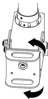
2. Rotate the head clamp 90° and insert the 4 screws again using the supplied 2.5mm Allen Key.
