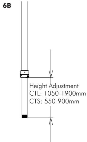
Slide Pole Assembly to the desired height.
