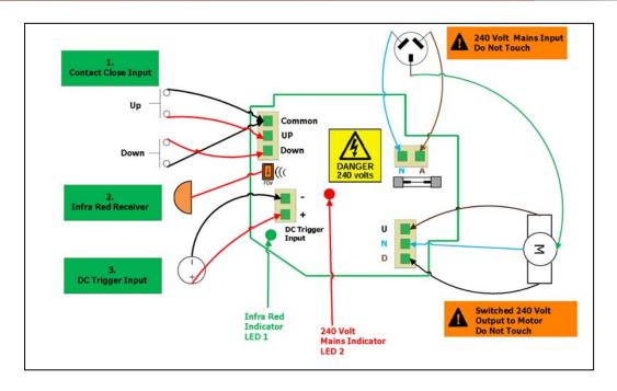
Access to control board is on left hand side of projector screen case Power must be removed before accessing inputs on control board
