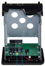
RAID mode DIP switches Set RAID button
