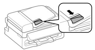
Insert the originals face-up and short edge first into the Automatic Document Feeder.
