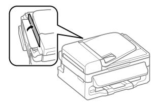
Slide out the paper support and the output tray and then raise the stopper.
