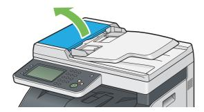
Remove the jammed document by carefully pulling it in the direction of the arrow shown in the following illustration.
