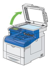
Place the document face down on the document glass and align it with the registration guide on the top left corner of the glass.
