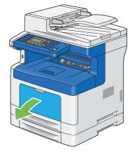
4 Grasp both sides of the bypass tray, and then pull the bypass tray from the printer.
