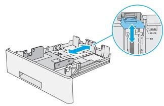
Load the paper into the tray. Make sure that the stack is flat at all four corners and that the top of the stack is below the maximum-height indicators.
