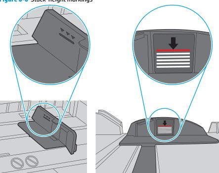
Figure 6-7 Tab for the paper stack
