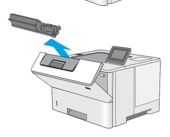
**4.** Lift the jam-access cover and slowly remove any jammed paper. Be careful not to tear the paper.
