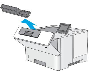
5. Lift the jam-access cover and slowly remove any jammed paper. Be careful not to tear the paper.
