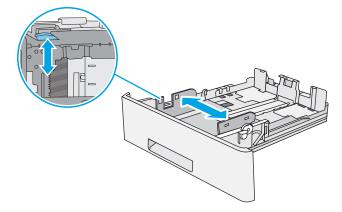
Adjust the paper-length guide by squeezing the adjustment latch and sliding the guide to the size of the paper being used.
