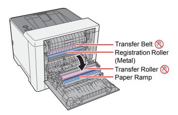
Wipe away the paper dust on the registration roller and the paper ramp using the cloth.
