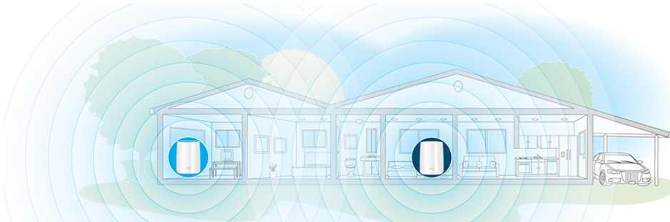
Figure 2. Single-story house with the Orbi satellite placed in the center
