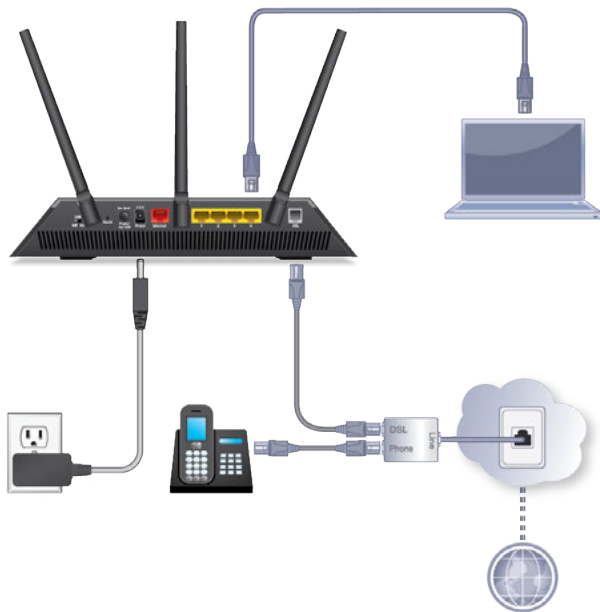
Figure 6. Modem router cabling for DSL service
