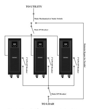
Fig. 6-2 Parallel System Installation Diagram
