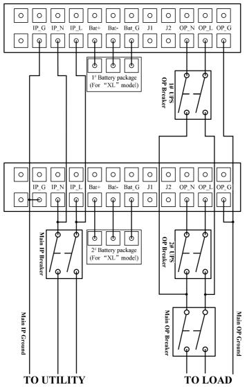
Fig. 6-1 Input and output Terminal Block wiring diagram
