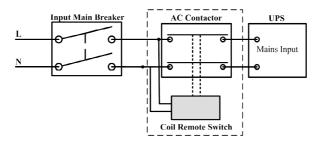
Fig.4-6 Typical external isolating device installation
