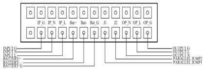
Fig. 4-7 Input and output Terminal Block wiring diagram
